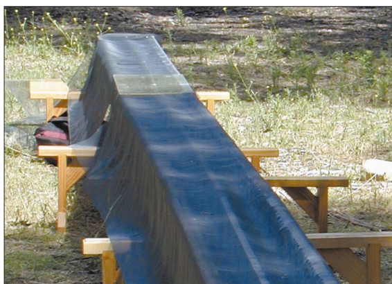
Figure 2. Closed at one end so the bees have only one point of entry, the tunnel is covered with black insect-screen cloth to permit observation and to give the bees a view of the sky. The test tunnel measures 6.4 meters long, 11 cm wide, and 20 cm high. (Photograph by Teresa Belcher, Research School of Biological Sciences, ANU.)
